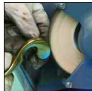
Polishing a brass door handle with a buffing wheel.
