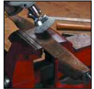
Removing rust from a lawnmower blade with a crimped wire cup brush.
