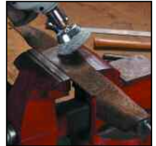
Removing rust from a lawnmower blade with a crimped wire cup brush.
